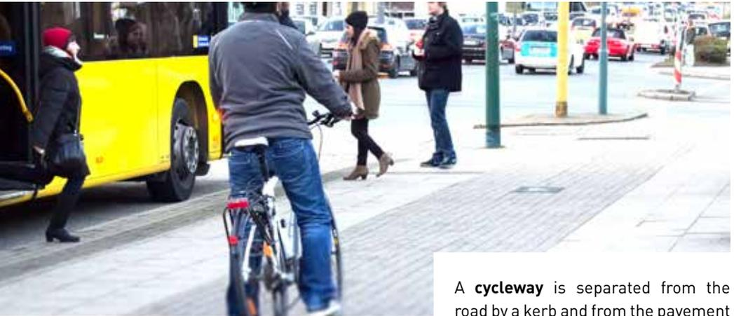
A **cycleway** is separated from the road by a kerb and from the pavement by markings, paving or a low kerb.
